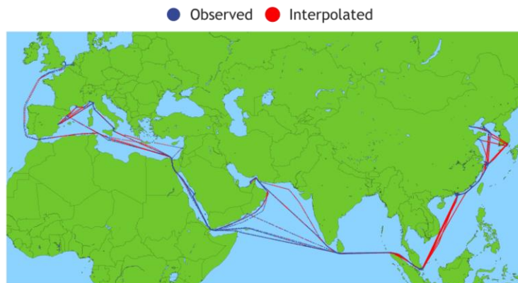
Figure 47 - A vessel's annual linearly interpolated ship activity, where 59% is represented by its observed activity and 41% is linearly interpolated
