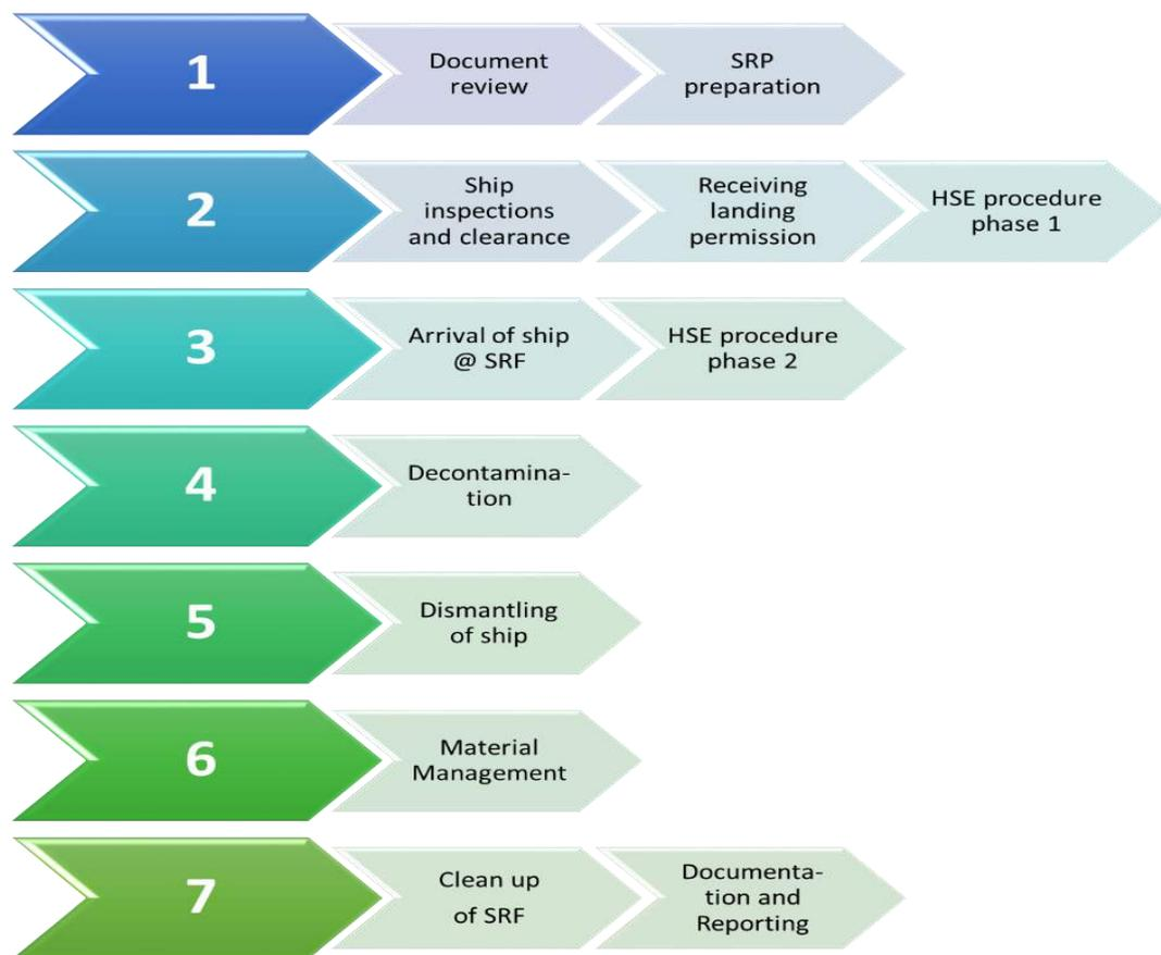
**Figure 7: Flow diagram of ship recycling**
