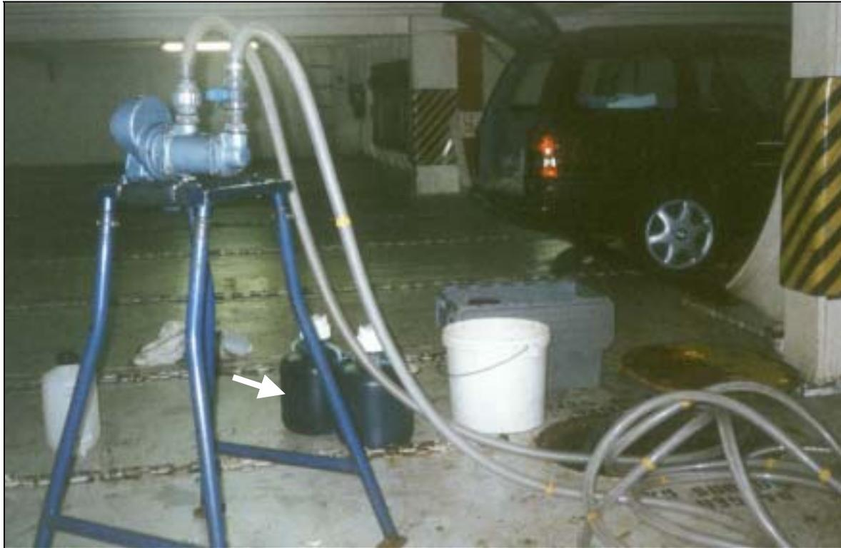
**Figure 1a.** Sampling equipment being used to collect sediment slurry (arrow) via ballast tank hatch from a double bottom tank of a car transporter.
