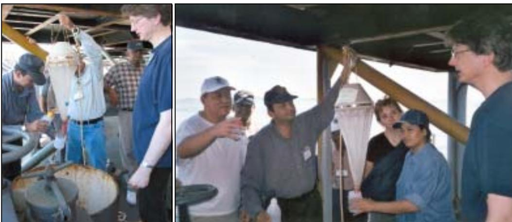
*German ballast water expert Dr Stephan Gollasch (right both pictures), demonstrating use of plankton nets lowered into the ballast tank via a manhole, aboard the Brazilian Navy tanker 'Marajo' (photos: A L Neto)*
