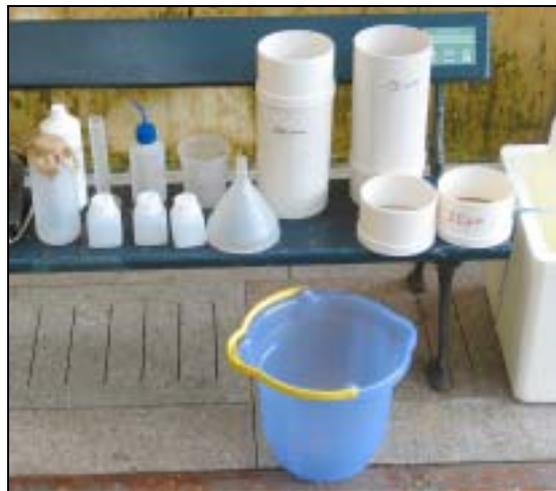
*Various accessories needed for shipboard ballast water sampling – including various sized sieves (right), sample bottles, plastic buckets etc (photo: A L Neto)*
