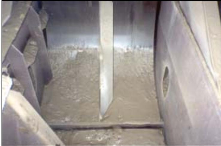
*Example of sediment accumulation in a ballast tank, requiring special sampling techniques (photo: D Oemcke)*
