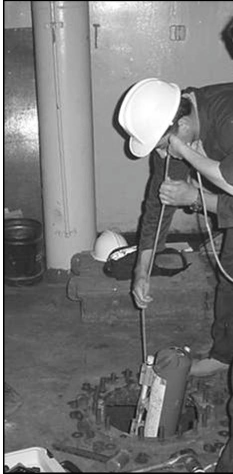
**Figure 1.** Sampling in the cement ship MARGRANEL by means of the opening of the tank.
