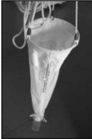
**Figure 5.** Plankton net (20  $\mu\text{m}$  mesh size) for concentrating water sample.
