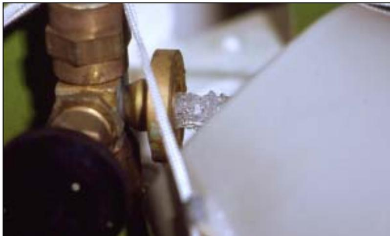
**Figure 5.** Water sampling at pressure meter of ships ballast pump.
