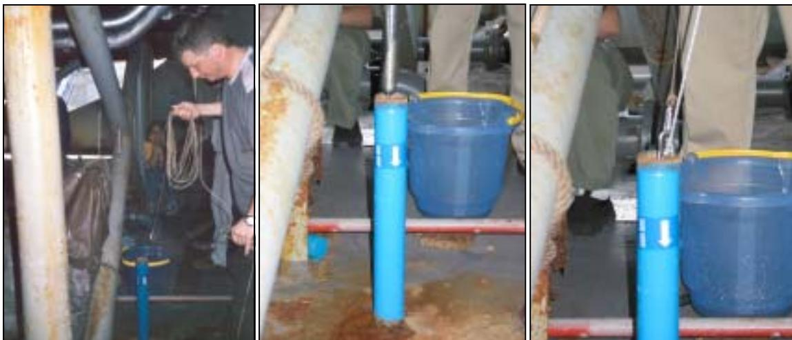
*Slovenian ballast water expert Matej David (left) demonstrating deployment of the bottom & sediment sampler via a sounding pipe aboard the 'Marajo' (photos: A L Neto)*
