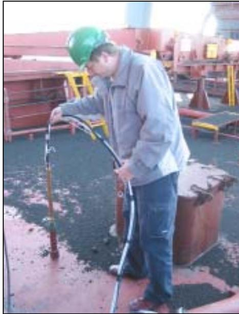
**Figure 1.** Shipboard sampling with the “Air-driven Well Pump”
