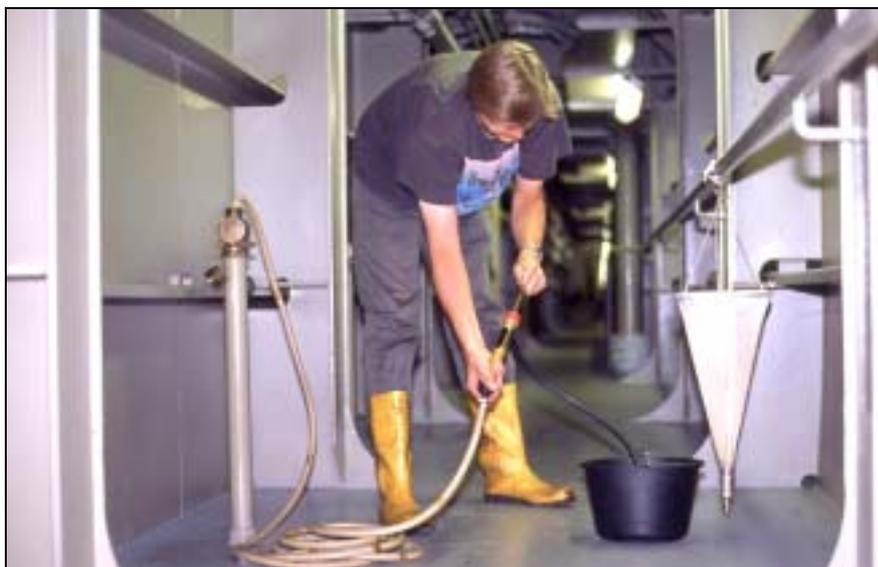
Figure 3. Ballast water sampling using a hand pump via sounding pipe.
