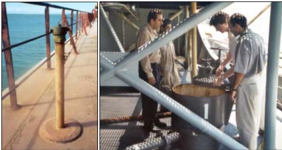
*Two points of access for ballast water sampling: Left – ballast tank sounding pipe (photo: D Oemcke); right – ballast tank manhole. Access via the sounding pipe is quicker, but is more restricted and less representative than via the manhole.*
