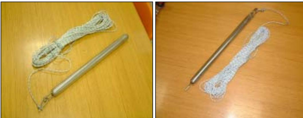
*The Slovenian 'Water-Column Sampler' (left) and 'Bottom and Sediment Sampler' (right) suitable for deployment via the ballast tank sounding pipe (photo: M David)*
