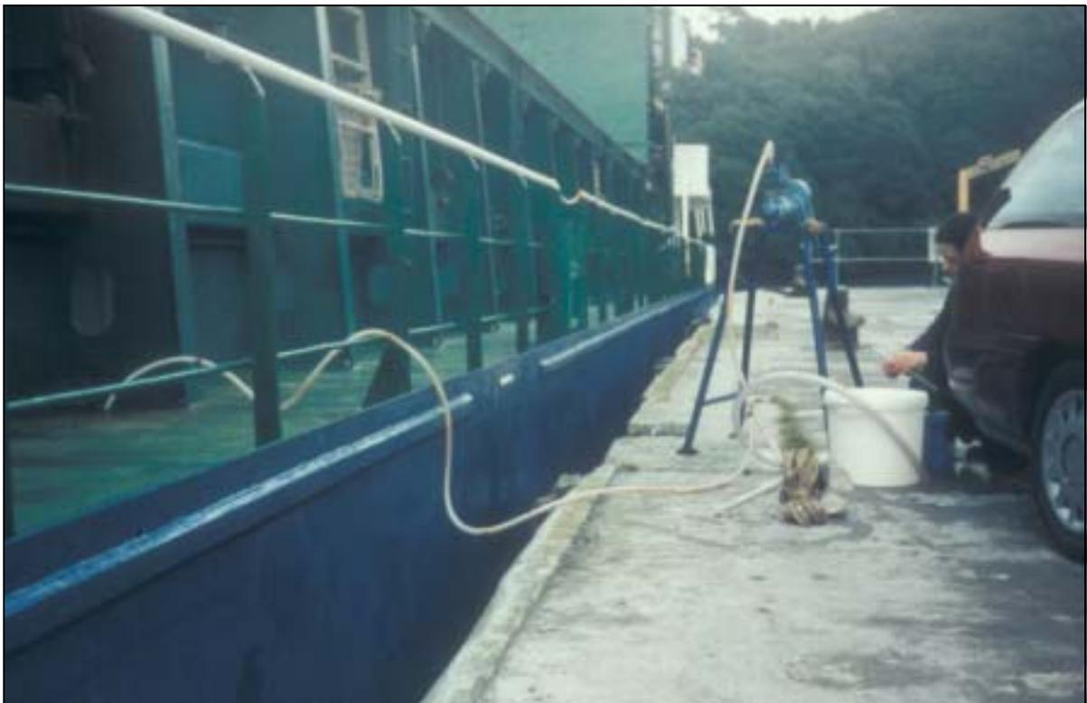
*Figure 1c & d. Reinforced hose pushed down a sounding pipe for collection of sediment slurry.*
