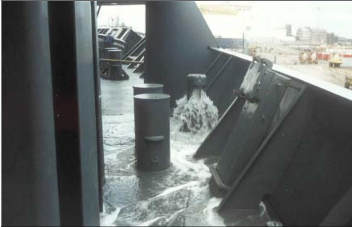
**Figure 1e.** Ballast tank being overflowed to allow collection of samples.
