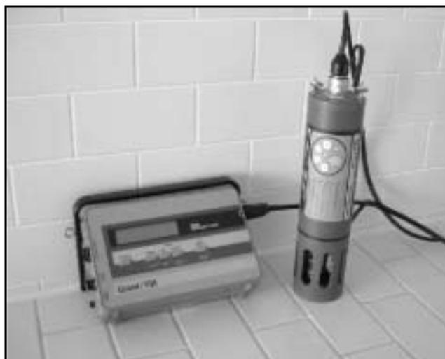
**Figure 2.** CTD meter for water quality sampling.
