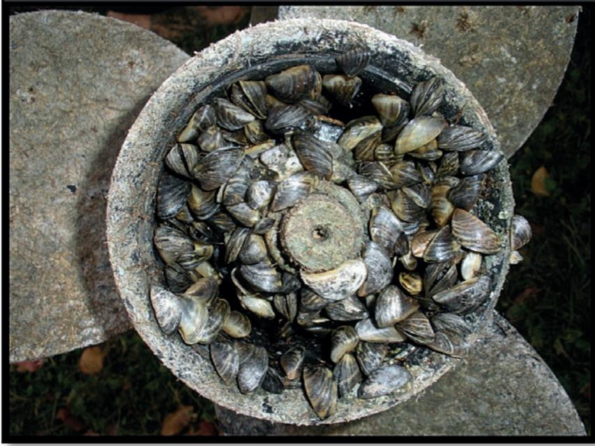
**Picture 6:** Zebra mussels attached to a boat propeller (Author: T. Britt - Source: *Flickr commons*).
