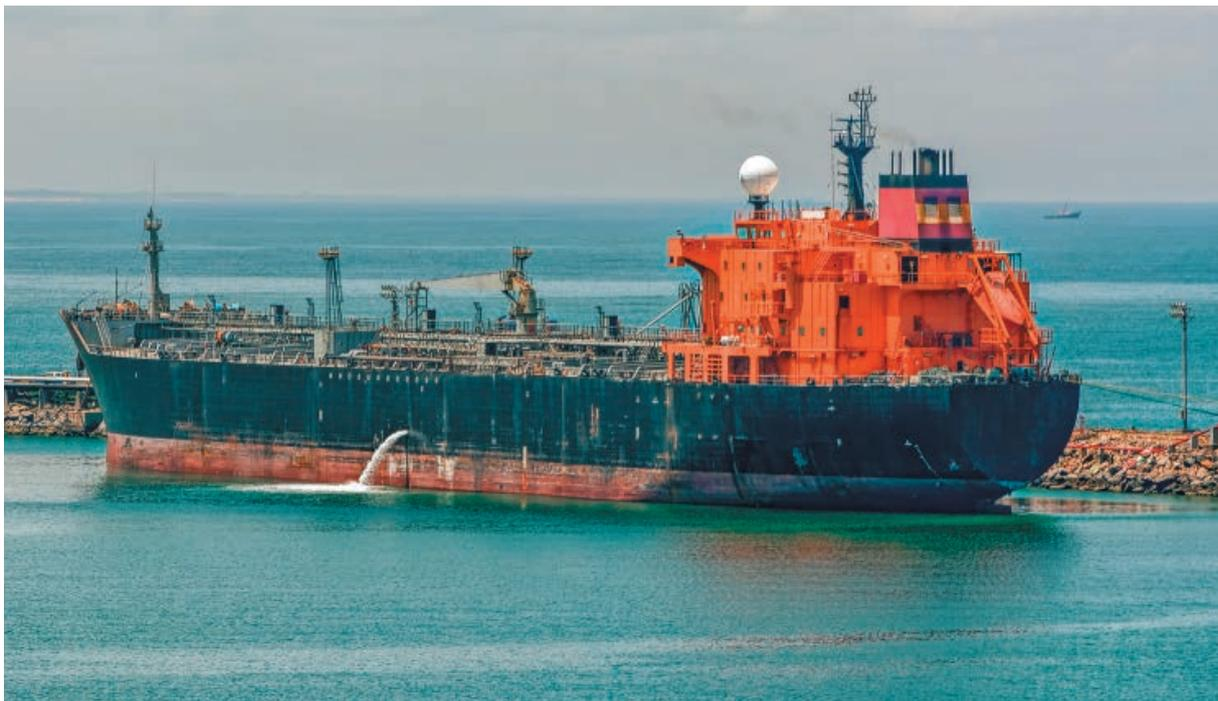
**Figure 1** Ship during ballast water operations, GloBallast.
