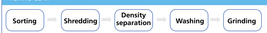
FIGURE 4. SCHEMATIC OVERVIEW OF THE PRE-TREATMENT PROCESSES FOR UNWANTED FISHING GEAR
