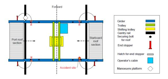
Figure 1: Simplified drawing of the gantry crane seen from above.
