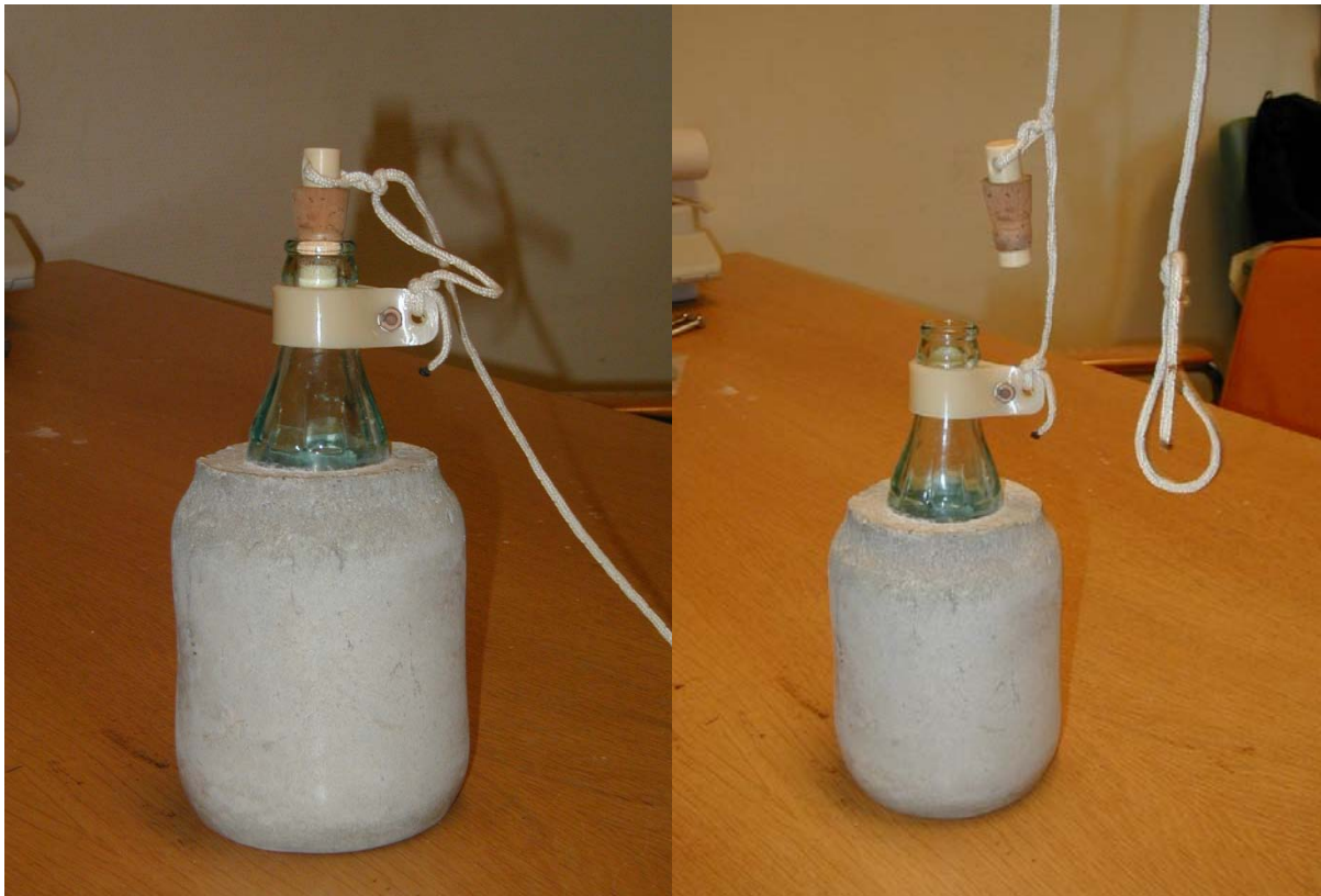
Figure 8. Cola Water Sample in the locked position and once released.
