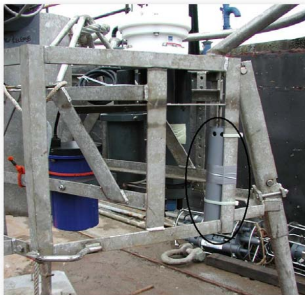
Figure 13. A Booner sediment trap (circled) mounted on a Cefas Seabed lander (MiniLander) and the design of a sediment trap.
