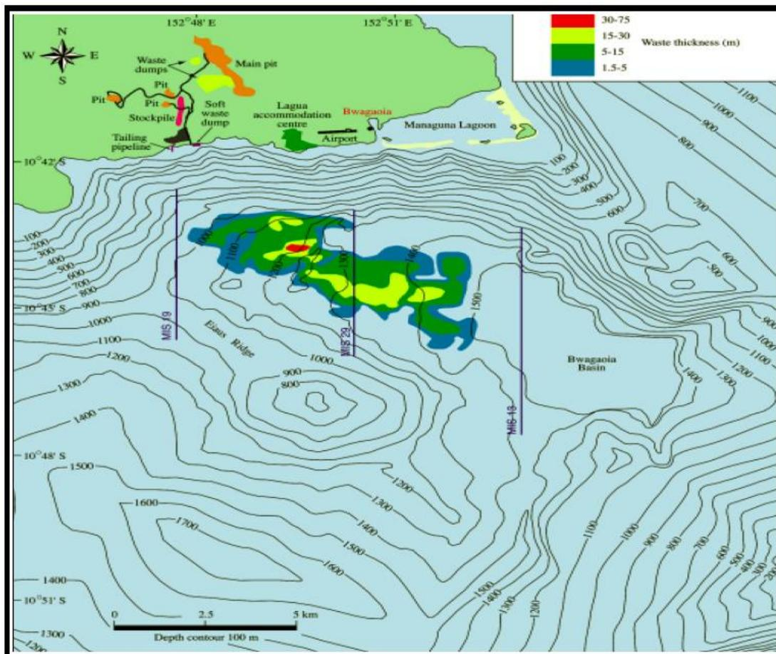
**Figure 15** Bathymetry of the Bwagaioia basin showing the area and thickness of tailings and soft waste deposition from Misima Mine (source: Shimmield 2010).
