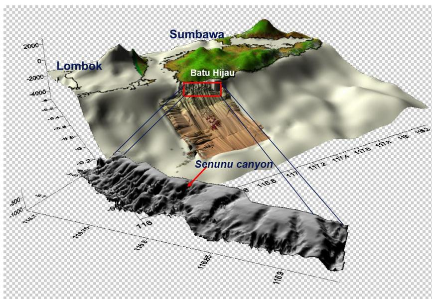
**Figure 12** Bathymetry at Batu Haju showing location of deep sea tailings placement into Senunu Canyon. Courtesy of Newmont Mining
