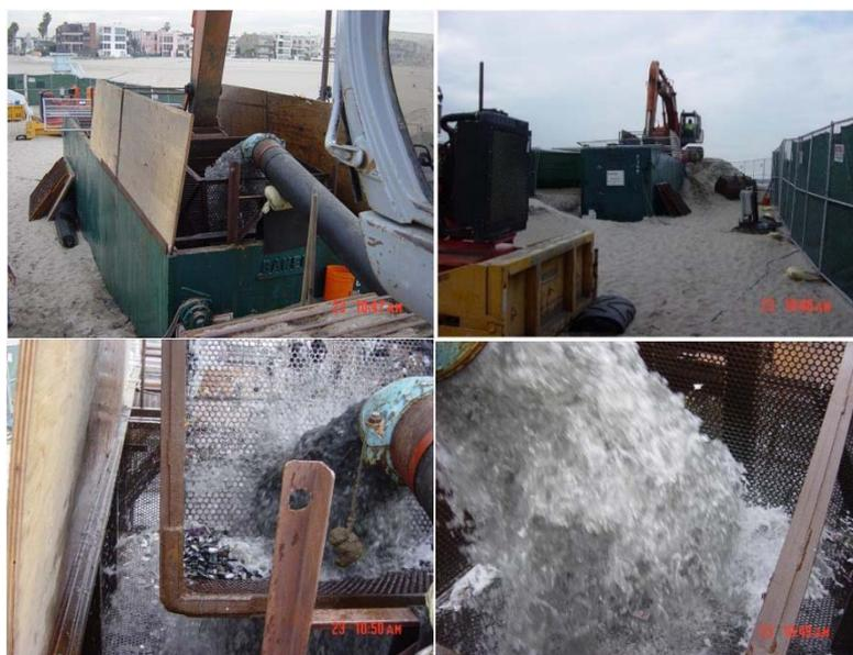
**Figure 11:** Separation of macrolitter from dredged material using a 1-inch mesh screening device attached to an 8-inch clamshell (Safra Altman from USACE ERDC Environmental Laboratory, personal communication)
