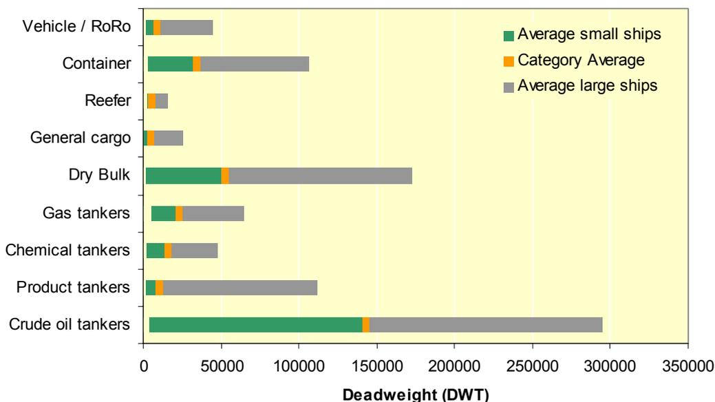
**Figure 2-6 – Deadweight of major cargo ship types. High and low end represent average deadweight of the upper and lower ship size categories that were used in the study, not of individual ships, which may be significantly larger or smaller [Lloyd’s Register – Fairplay, 2007]**
