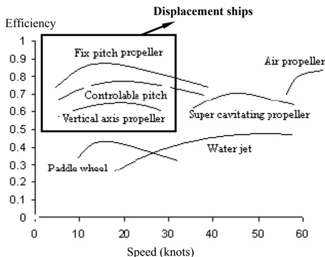
Figure A2-6 – Efficiency of propulsive devices [31]
