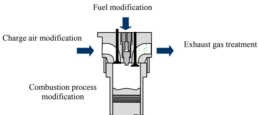
**Figure A2-6 – Ways to reduce NO<sub>x</sub> emissions from a marine diesel engine**
