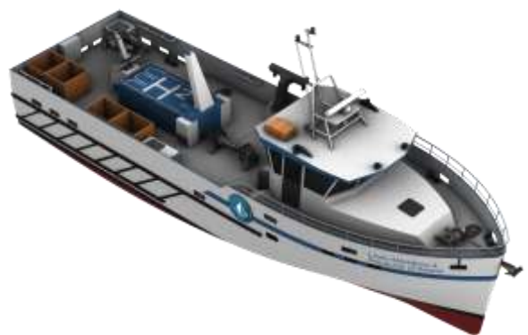
Hydrogen-powered fishing vessel (Credits: Mauric)
