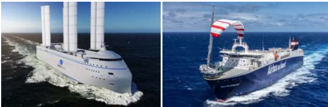
Example of wind propulsion systems under development (credits Ayro and Airseas)
