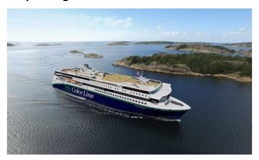
Color Line's new ship the Color Hybrid is to be delivered by the Ulstein shipyard next year, and will be the world's largest hybrid passenger ferry. It will operate on the Sandefjord-Strømstad crossing. It is being equipped with a 4.7 MWh battery pack which will allow it to sail 3.2 nautical miles on battery power alone. The ship will be charged using shore power during the overnight stay in Sandefjord. Photo: Fosen Yard/Ulstein
