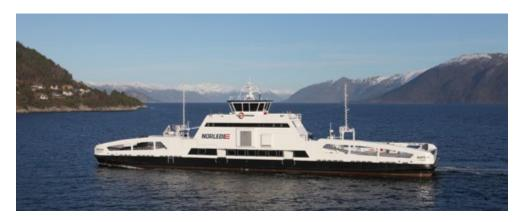
Since 2013, the *MF Ampere*, the world's first battery-propelled ferry, has provided a service across the Sognefjorden between Lavik and Oppedal. Photo: Norled
