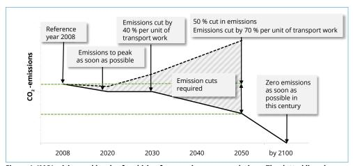
Figure 1: IMO's vision and levels of ambition for greenhouse gas emissions. The dotted line shows the projected emission trend under a business-as-usual scenario. The solid line shows an emission trajectory in line with IMO's strategy.
