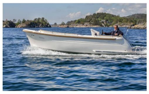
GreenWaves 601 is an all-electric Norwegian motorboat. The standard motor is 7.5 kW and the standard lithium battery pack allows 5–7 peaceful hours at sea. Photo: Johner Bildbyrå AB
