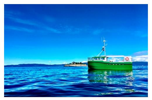
Karoline is the world's first hybrid fishing boat with an electric propulsion system. The vessel is 11 metres long, and has a diesel engine for use to and from the fishing grounds. The battery packs provide the vessel with enough power for two hours fishing and 45 minutes of propulsion. Photo: SIEMENS
