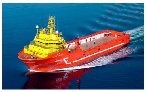
Eidesvik's supply vessel *Viking Energy* was launched in 2003 as the first LNG-powered offshore vessel. The ship made history again in 2016, when it was fitted with an advanced battery system that has reduced annual fuel consumption by 17 %. The battery system has a capacity of 650 kWh/1600 KW. Photo: Eidesvik Offshore
