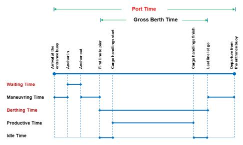
Figure 2.3 - Breakdown of ship's time in port
