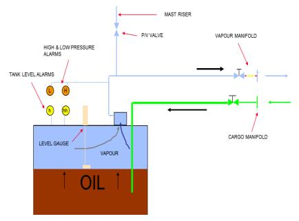
Figure 6.1 – Schematic of an oil tanker's VOC emissions control system
