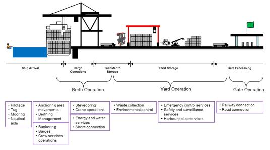
Figure 2.4 - Schematic diagram of container terminal operations with activities
