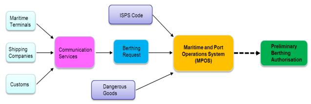
Figure 2.5 - Application of berthing request in a typical port management system
