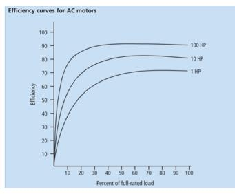
Figure 6.6 – Typical characteristic of electric motors [6]
