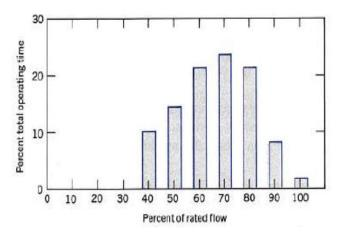
Figure 6.3 – Load profile for a typical pump
