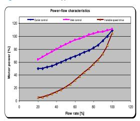
Figure 6.5 – Impact of Variable Speed Drive method of flow control on power demand
