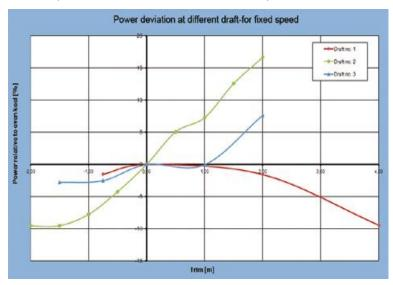
Figure 3.4: Trim guidance at different drafts [Force Technology 2011]
