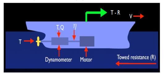
Figure 3.2: Schematic of parameters measured under model self-propulsion tests [Rod Sampson 2008]
