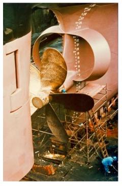
Figure 9.2 – Typical wake equalising duct [Scheneekluth]
