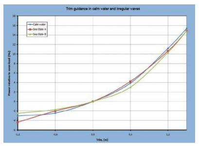
Figure 3.5: Impact of waves relative to calm waters [Force Technology 2011]
