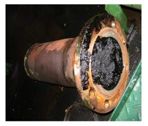
Figure 7.1 - Clogged fuel pipes due to very poor quality fuels
