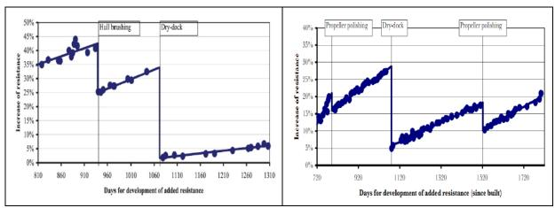
shows typical ship increased resistance as a function of time and impact of hull surface improvements due to maintenance efforts.
