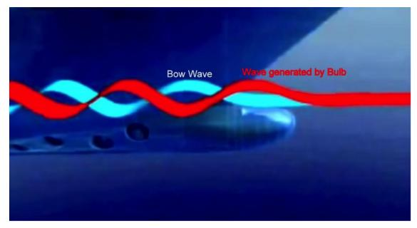
Figure 9.8 - Concept of bow waves and bulb waves that cancel each other [Soumya Chakraborty]
