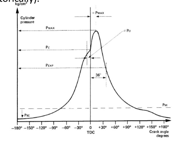
than expected cylinder pressure Lower generally means that engine settings are not optimal or its components may be faulty. In practice, other engine process parameters such as pressures, temperatures, turbocharger
