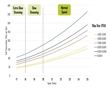
**Figure 3.3 – Ship fuel consumption dependence on ship speed** [Geography of Transport System, adapted from Notteboom et al (2009)]
