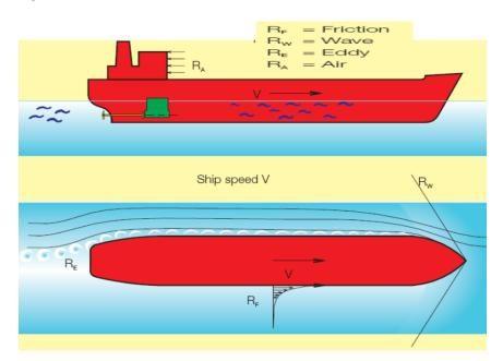
Figure 3.1 shows a schematic of these resistances.
