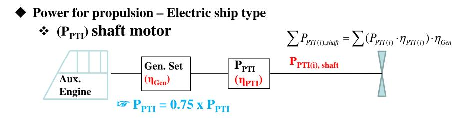
Measurement of V<sub>ref</sub> (main engine + shaft motor)
