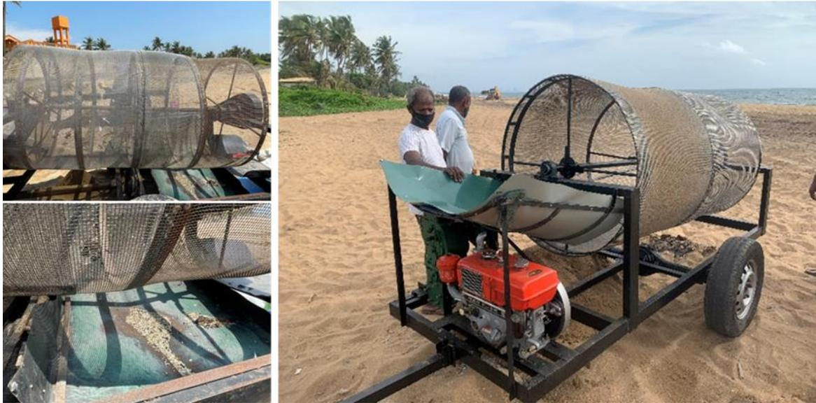
**Figure 20:** Mechanical trommels. Source: ITOFF.
