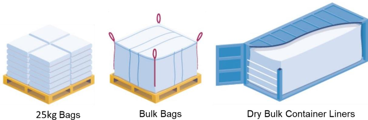
**Figure 4:** Types of plastic pellet packaging. Source: ITOFF
