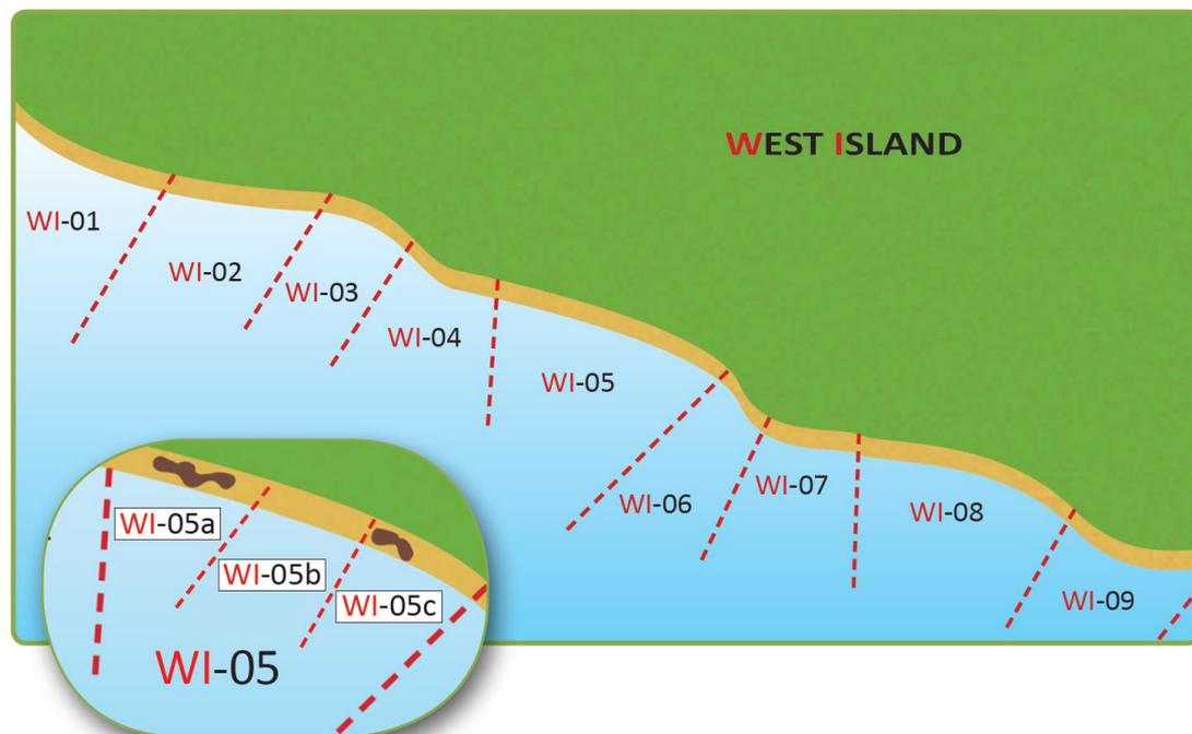
**Figure 12:** Example of subdivision of a coastline into segments assigned a unique ID. Source: Oil Spill Response Limited, SCAT Field Guide<sup>27</sup>.
