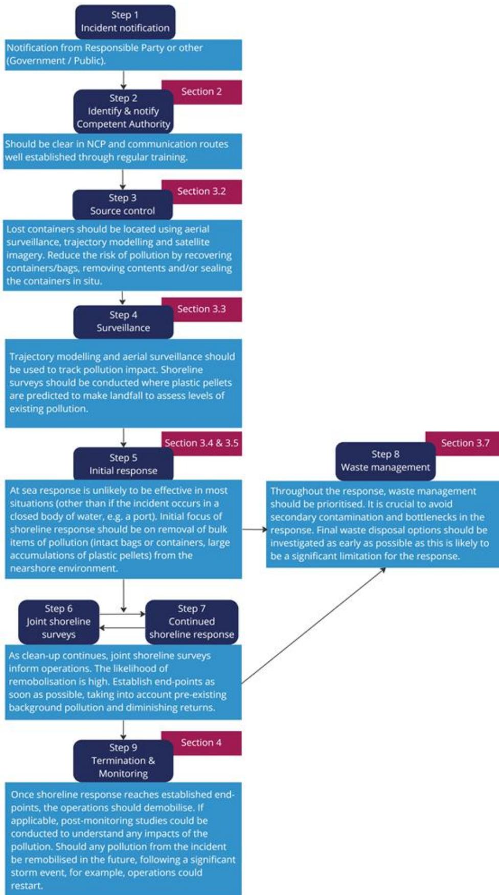
**Figure 1:** Flowchart to illustrate typical steps to take following a ship-source plastic pellet spill, with reference to sections of this document for further information.
