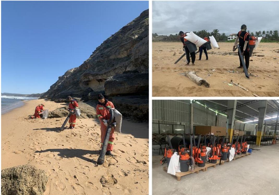
**Figure 19:** Vacuum recovery units. Source: ITOPF.
