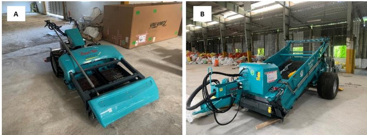
**Figure 22:** Different types of beach cleaners. A) walk-behind; B) tractor drawn. Source: ITOPF.
