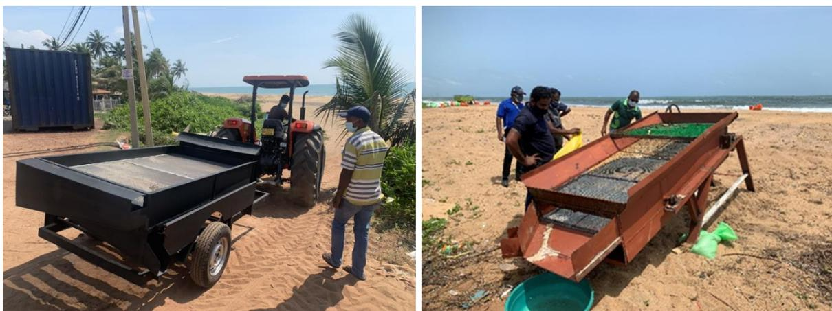
**Figure 21:** Mechanical table screeners. Source: ITOFF
