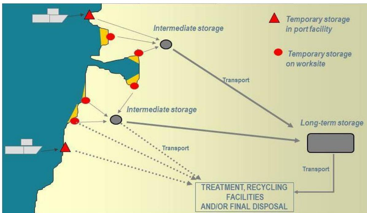
**Figure 25:** Waste storage and transport options between spill sites and treatment or disposal facilities<sup>34</sup>.
