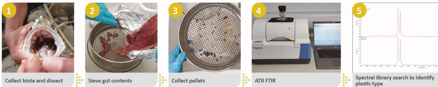
Figure 33: Illustration of workflow for characterisation of plastic type. Source: Cefas
