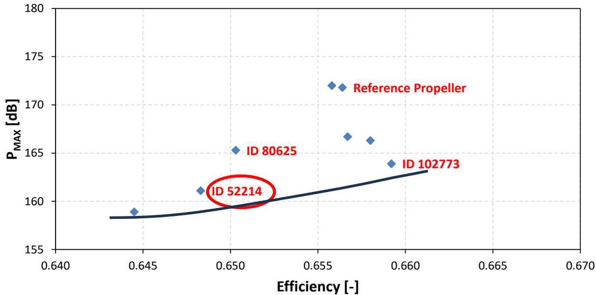
ETV calculations (maximum vortex peak pressure vs propeller efficiency for different propellers)
