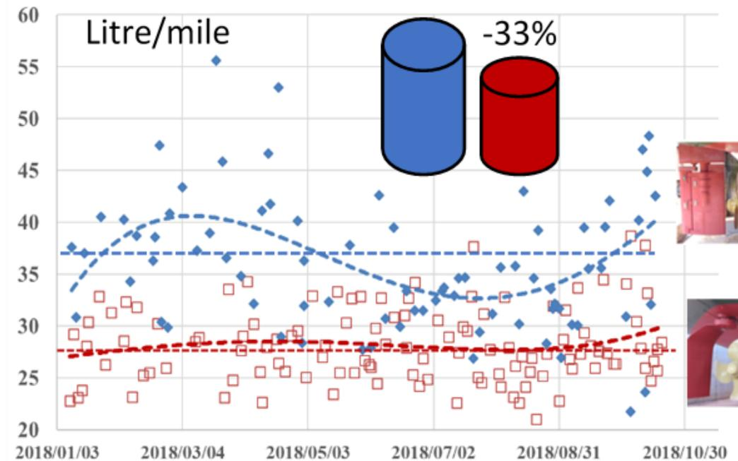
**Trials** (calm water) and in-service (including rough weather) powering performance comparisons of two sister ships: one **Shigenobu** with Gate rudder system **vs. Sakura** with Conventional flap-rudder system
