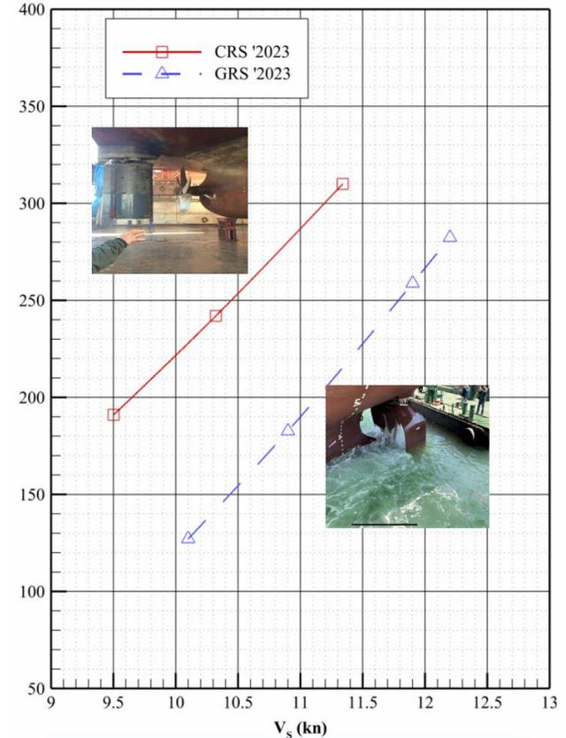
Measured Fuel Consumption comparison of MV ERGE before and after GRS retrofit in trials (2023)
