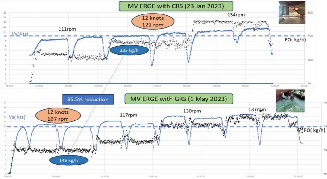
Measured Fuel Consumption comparison of MV ERGE before and after GRS retrofit in trials (2023)
