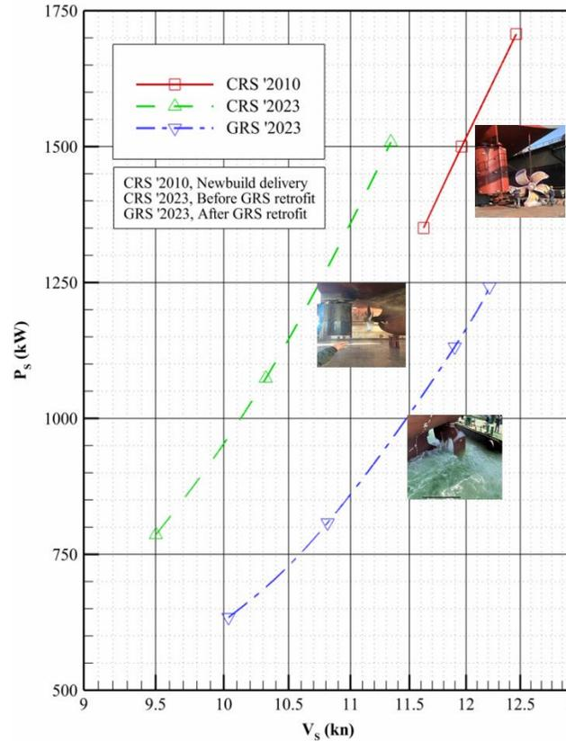
Measured trial shaft power ( $P_s$ ) comparison of MV ERGE before and after retrofit in the present (2023) and when she was new (2010).
