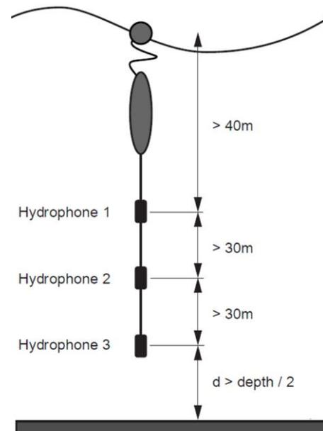
Three hydrophones have been used deployed at three different water depths, at 40, 70, and 100 meter tethered from a support vessel. The three hydrophones were connected to the RTSYS EA-SDA14 data recorder which has been set to sample the hydrophone signal at a sampling frequency 156.25 kHz (24 bit).
