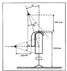
Test set-up for test of automatic inflation system
