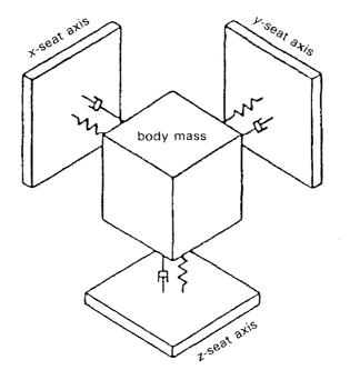
Figure 3 - Independent single-degree-of-freedom representation of human body
