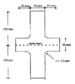
Figure 1 Sample specification for sewn canopy seams
