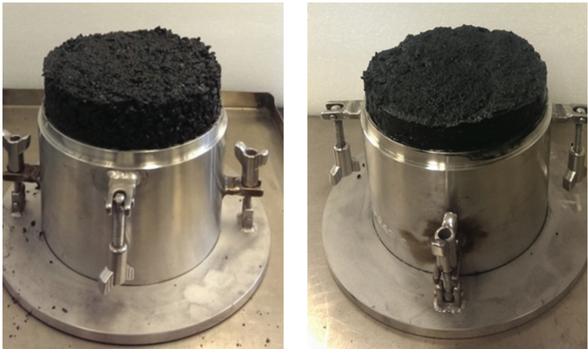
Figure 1.5.5.3.4.1 – Photographs showing valid tests for a partially saturated test portion (left) and a near fully saturated test portion (right)
