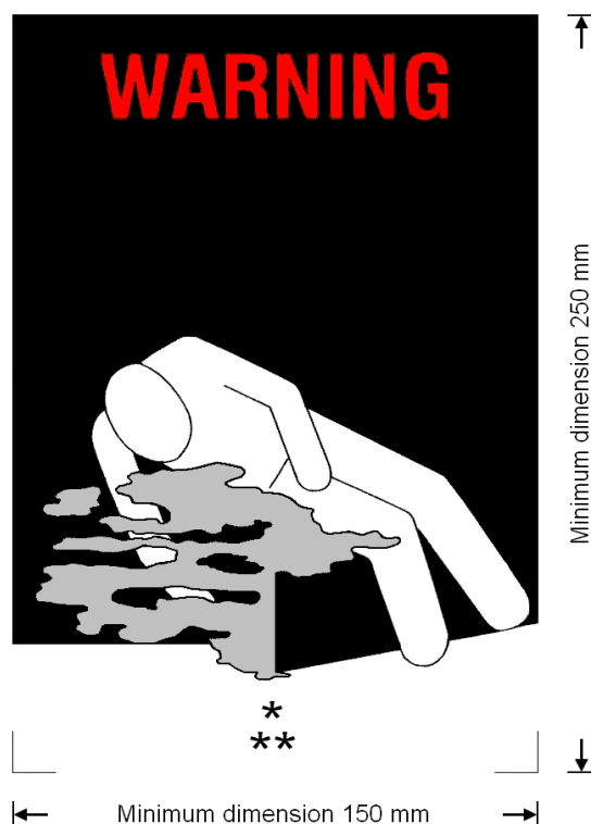
Coolant/conditioning warning mark for cargo transport units
