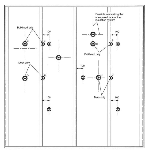
Thermocouples used for maximum temperature rise and in calculating average temperature rise.
