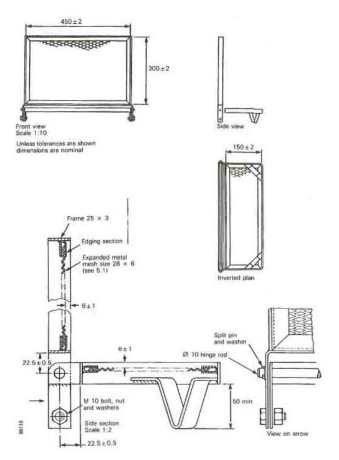
Figure 1 – Test rig (All dimensions are in millimetres. All parts are of steel.)
