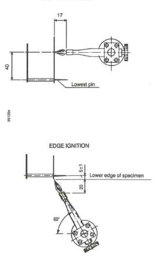
Figure 2 – Ignition burner: fabric positions
