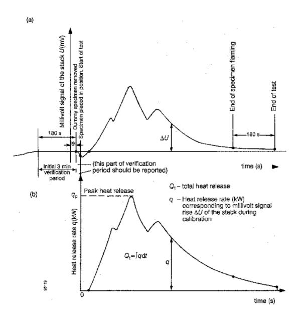
Figure 10 – Example of conversion of the millivolt signal rise ΔU to heat release rate of the specimen
