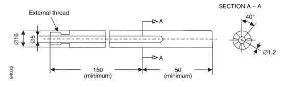
Figure 5 – Pressure-sensing heads
