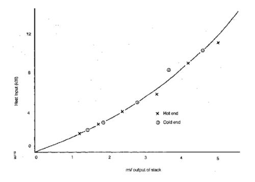
Figure 9 – Example of a typical stack calibration
