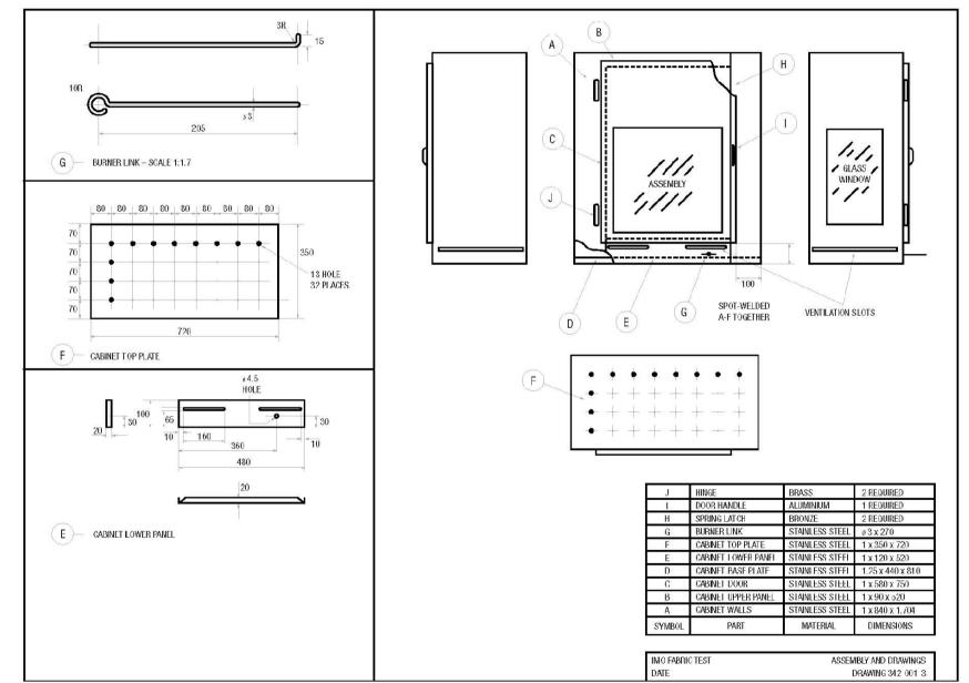
Figure 5 – Fabric test: test enclosure
