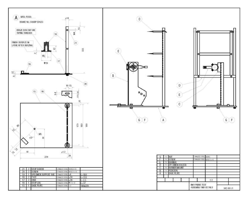
Figure 3 – Fabric test: assembly and details
