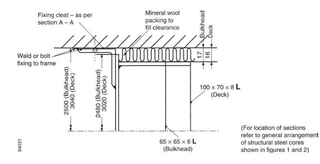
Figure 3 – Connection between restraint frame and structural steel core
