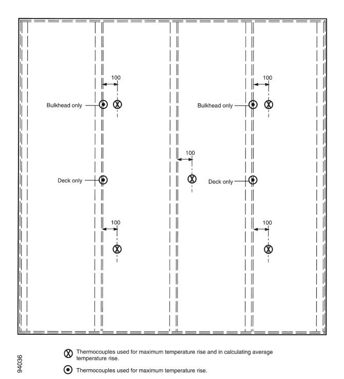
Figure 8 – Position of unexposed-face thermocouples for "A" class division: flat face of structural steel core to the laboratory RESOLUTION MSC.307(88) (adopted on 3 December 2010) INTERNATIONAL CODE FOR APPLICATION OF FIRE TEST PROCEDURES, 2010 (2010 FTP CODE) - 67 -
