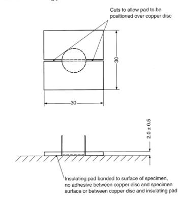
Figure 6 – Unexposed-surface thermocouple junction and insulating pad
