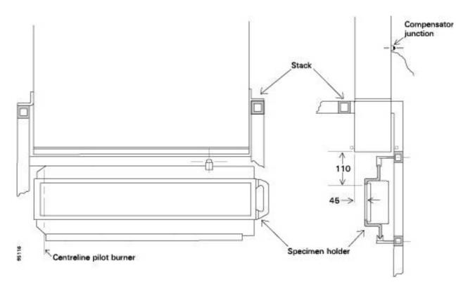
Figure 4 – Position of stack and specimen
