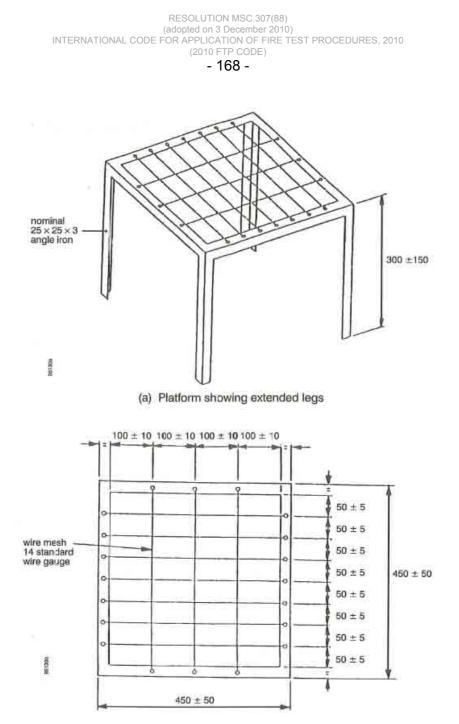
(b) Spacing of wire mesh platform
