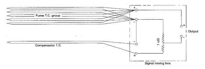
Figure 7 – Diagrammatic sketch of thermocouple circuit
