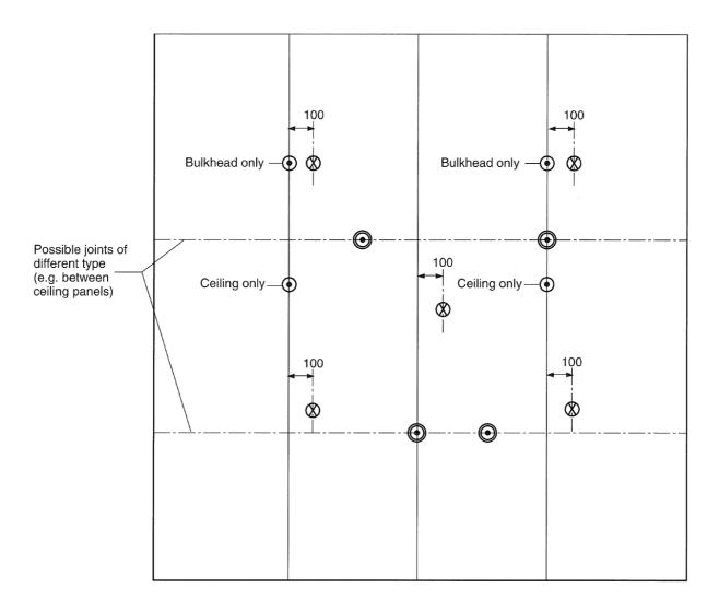
Thermocouples used for maximum temperature rise and in calculating average temperature rise.
