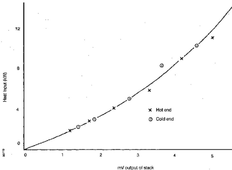
**Figure 9 – Example of a typical stack calibration**
