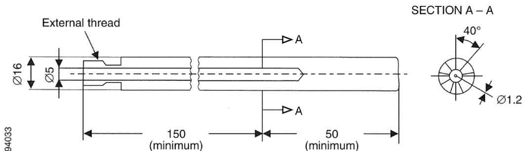
**Figure 5 – Pressure-sensing heads**
