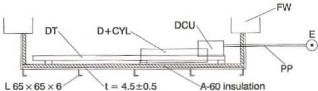
D = door model, DCU = door control unit, DT = door track, WF = weld fastening, GT = guide track, CYL = door cylinder, R = supporting roller, PS = piping systems, PG = pressure gauge, PP = pressure pipe, E = Energy, FW = furnace wall.
