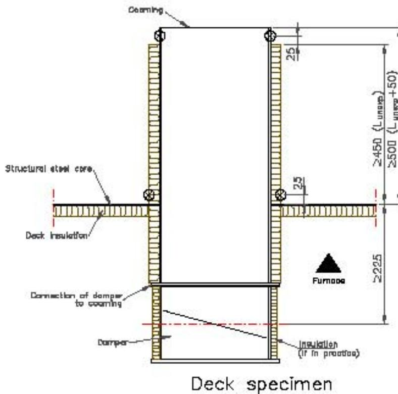
$L_{unexp}$  = Needed insulation length for a damper under a test
