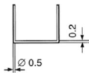
When making the junction of the thermocouple wires to the copper disc, a minimum amount of solder shall be used for the purpose. Any surplus solder shall be removed.
