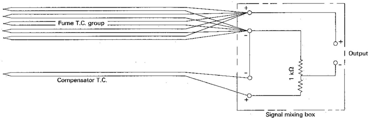
Figure 7 – Diagrammatic sketch of thermocouple circuit
