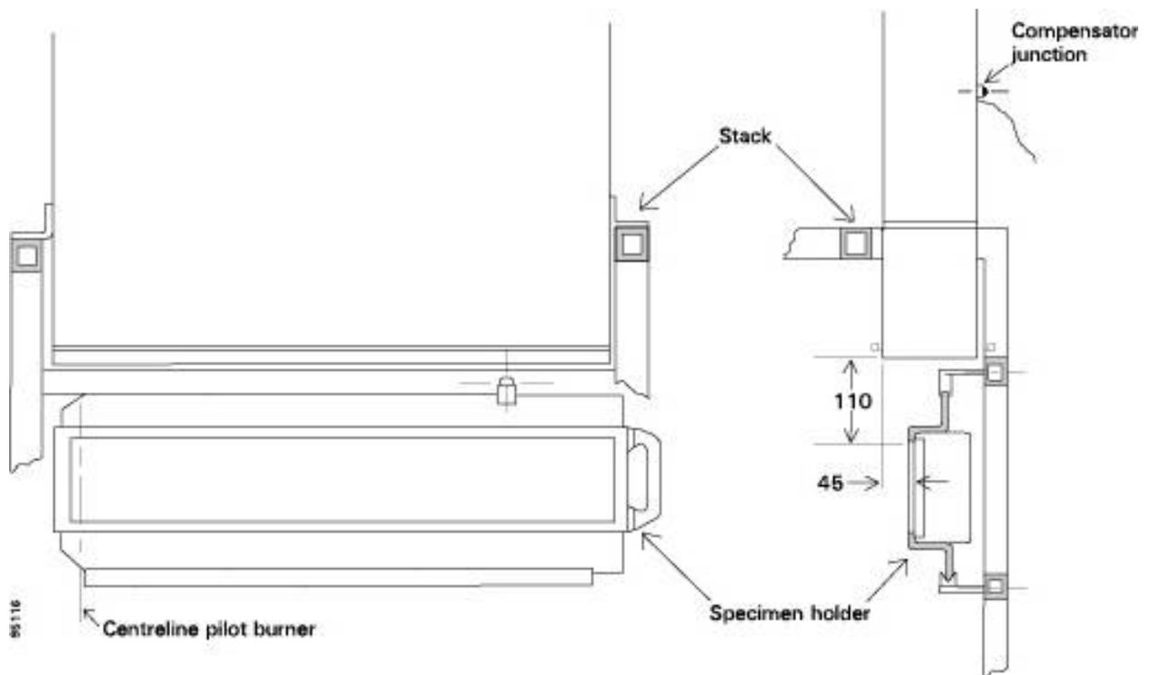
Figure 4 – Position of stack and specimen
