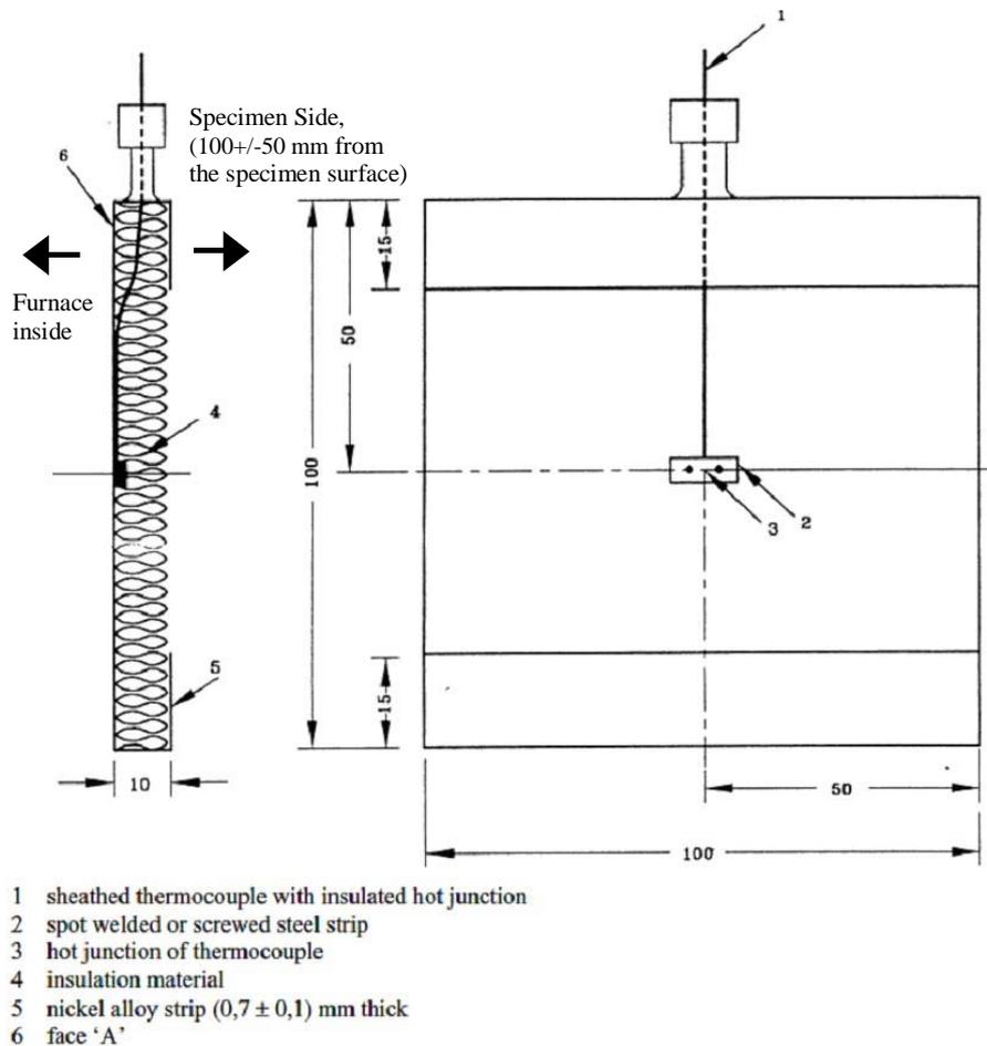
**Figure 4 – Furnace thermocouple assembly**
