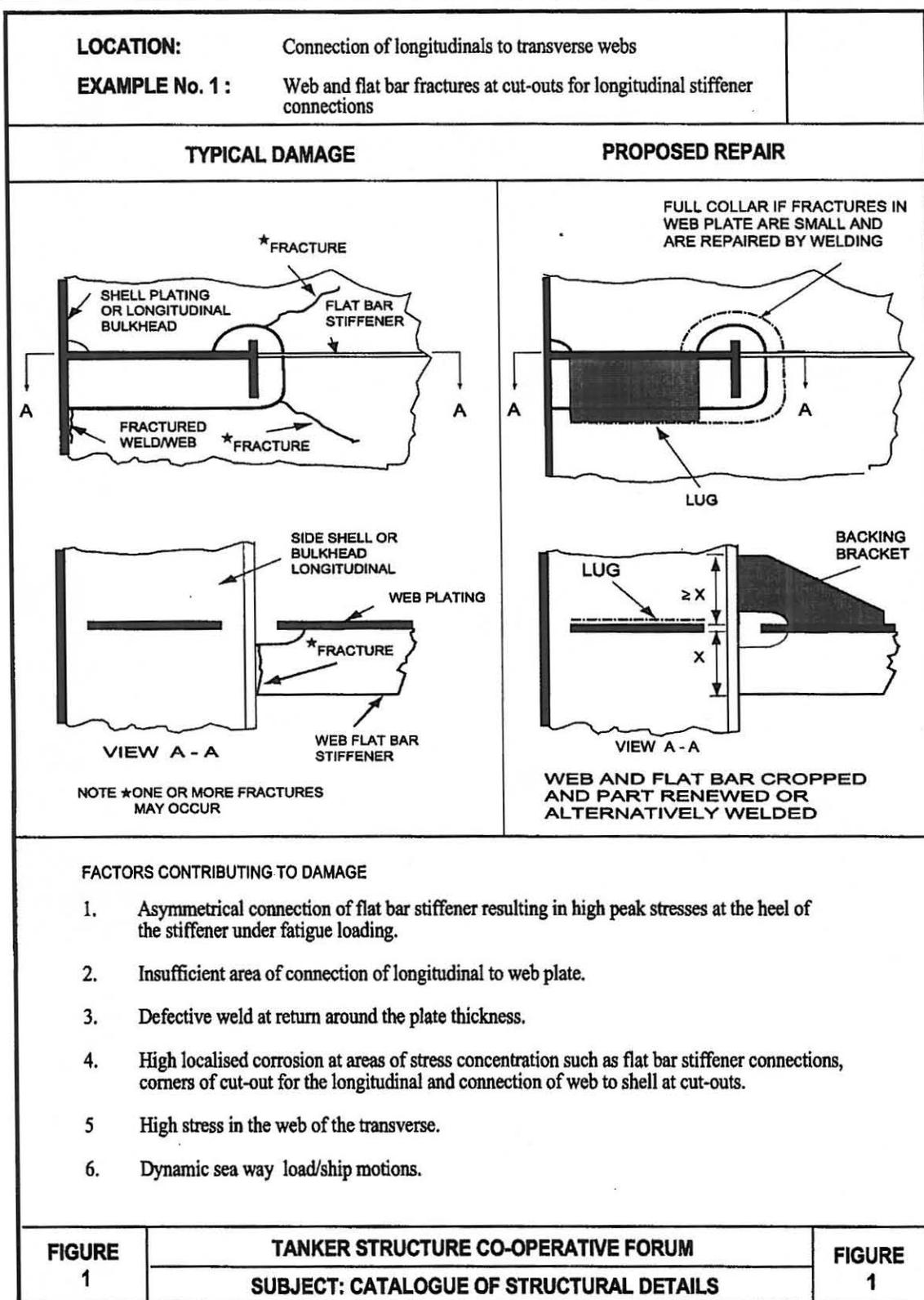
**FIGURE 2: TYPICAL DAMAGE AND REPAIR EXAMPLE
