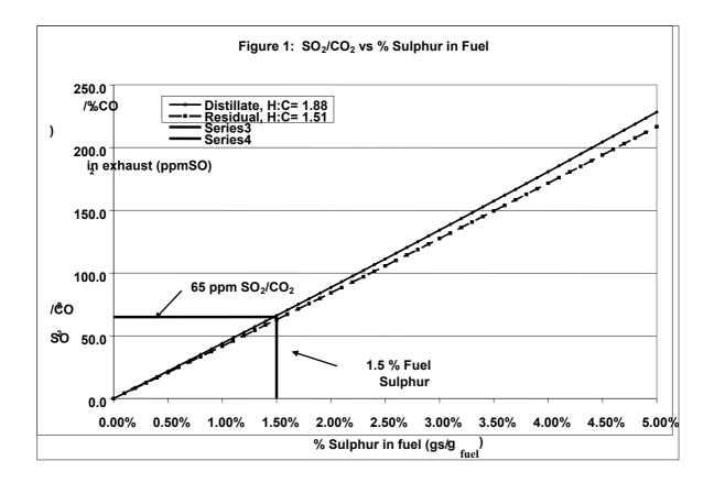
Correspondence between 65 (¹ppm/%) / CO<sub>2</sub> and 6.0 g/kWh is demonstrated by showing that their S/C ratios are similar. This requires the additional assumption of a brake-specific fuel consumption value of 200 g/kWh. This is an appropriate average for marine diesel engines. The calculation is as follows:
