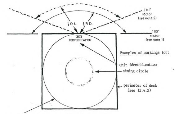
deck size as declined by overall length (O L) or rotor diameter (RD) as appropriate (see 13.2.2 and 13.2.3)
