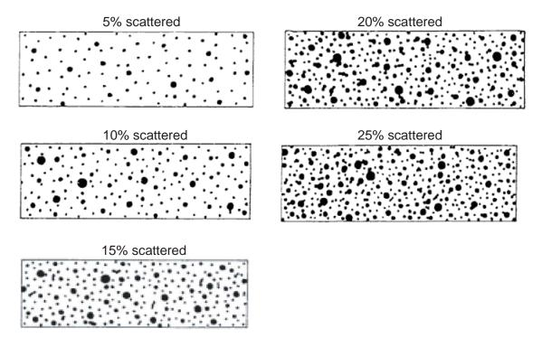
Figure 2 – Pitting intensity diagrams (from 5 to 25% intensity)
