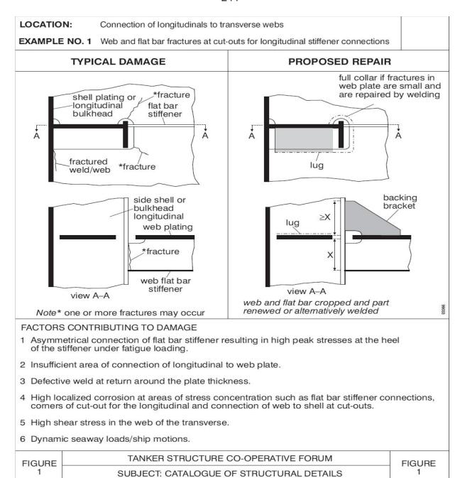
Figure 2 – Typical damage and repair example (reproduced from reference 2)
