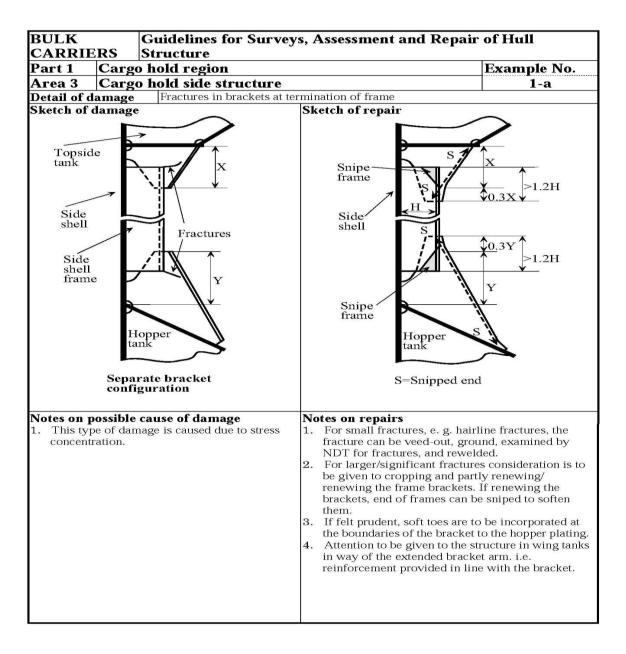
Figure 3 – Typical damage and repair example (reproduced from reference 3)
