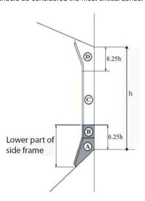
Figure 1 – Zones of side shell frames and brackets
