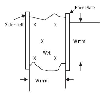
Figure 3 – Typical five-point pattern on the web plate
