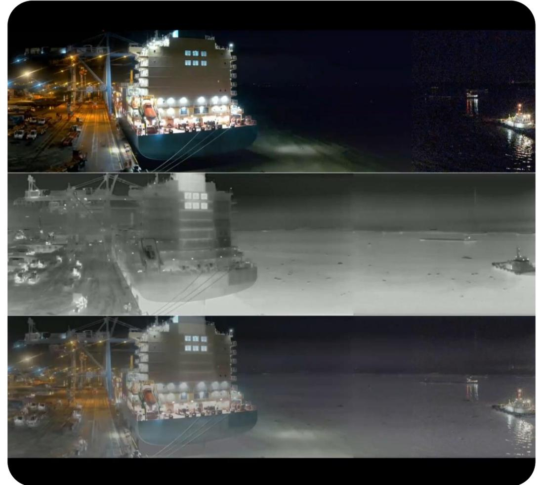
**Sensor fusion technology enhances accuracy** by complementing individual sensor strengths and weaknesses, providing a more complete understanding of the situation.
